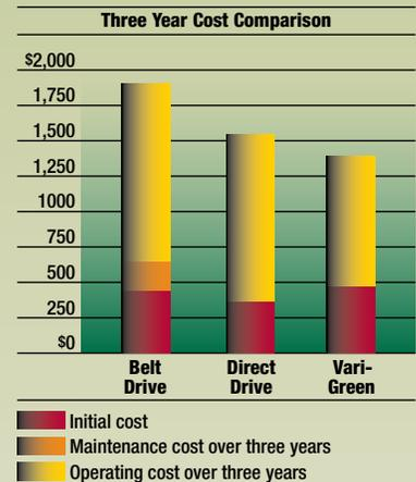
Analysis is based on operating costs for a period of three years where the fans operate continuously at 1725 rpm, 24/7, with an energy rate of \$0.10 kWh. Maintenance on the belt drive is estimated at \$65/yr. Note: Example is based on a relative cost. Use and installation variables may produce different results.
